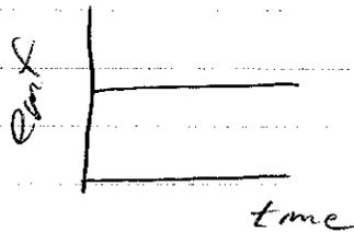
$$\begin{aligned}\textcircled{3} \quad \mathcal{E} &= -N \frac{\Delta \Phi}{\Delta t} & \Phi &= BA \cos \theta \\ &= -N \frac{BA \cos \theta_2 - BA \cos \theta_1}{\Delta t} \\ &= -950 \frac{(8.56 \times 10^{-5}) (\pi (.06)^2) (\cos 45 - \cos 0)}{\Delta t} \\ &= \underline{2.7 \times 10^{-3} \text{ V}}\end{aligned}$$
